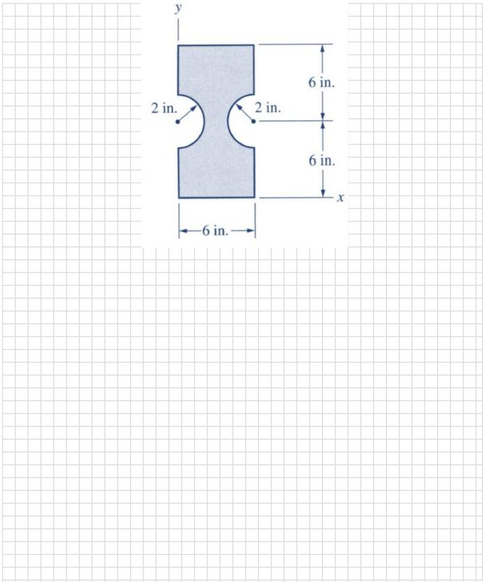
8-28. 8-26 to 8-31 For each built-up section shown in Figs. P8-26 to P8-31, determine the moment of inertia and the radius of gyration of the section with respect to the horizontal centroidal axis. Solution.
